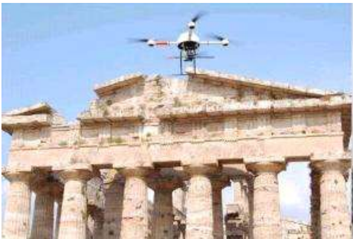
Figure 5- Use of MD4-1000 for aerial suvey.
